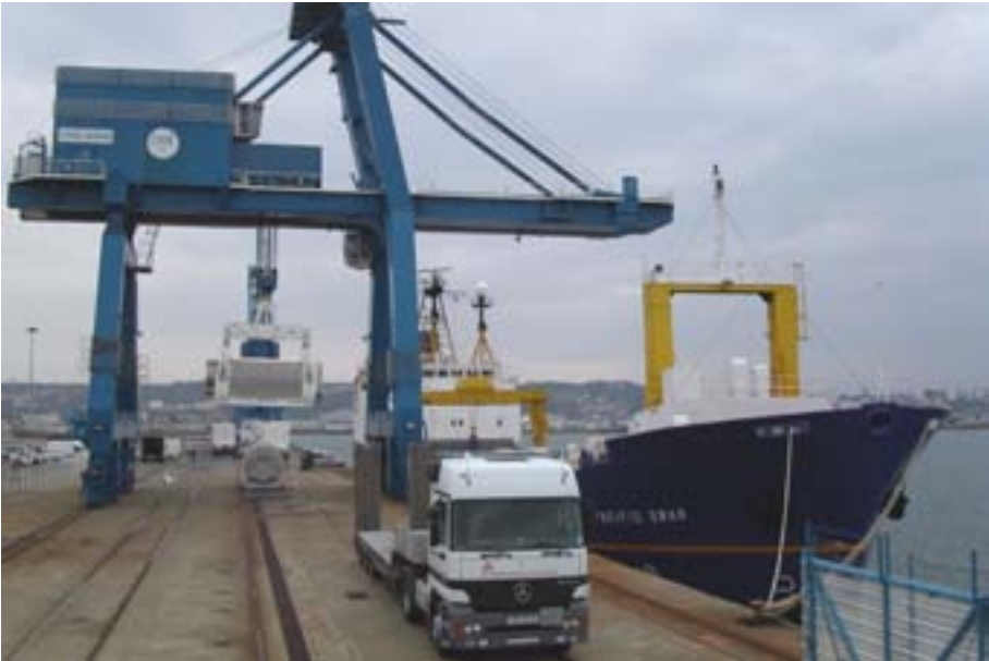
FIG. 12. Unloading a vitrified waste cask from a truck and loading it on to a ship at the port of Cherbourg.
