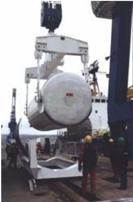
FIG. 14. Vitrified residues: cask for shipment to Japan, Belgium and the Netherlands.
