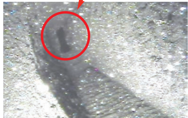
Illustration of clogging of the foliate channels on a steam generator tube support plate
