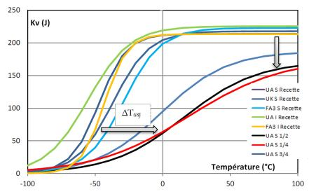
Figure 27: Comparison of transition curves in segregation zone by comparison with the acceptance zone for the UA Upper dome with the highest carbon content
