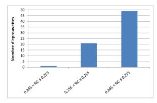
Figure 39: Carbon content of toughness specimens tested in the ductile domain
