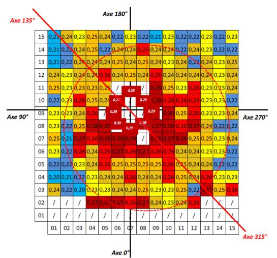
Figure A20 : Illustration of the most segregated zone on external surface of UA upper dome (IRC measurements) Measurement pitch 50 mm x 50 mm
