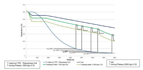
Figure A7: Characterisation of the hot shock caused by the RCN further to a small break in the primary cooling system
