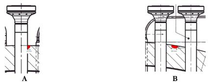
Figure 47: Flaws simulated for the ultrasounds inspection
