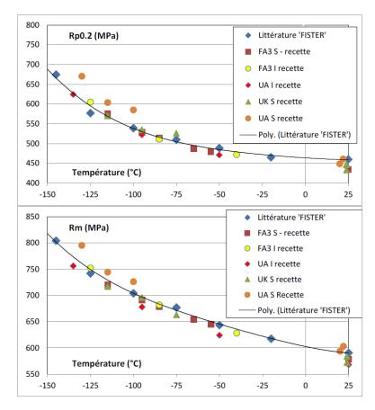
Figure 25: Evolution versus temperature of the yield strength  $R_{p0.2}$  (top graph) and ultimate tensile strength  $R_m$  (bottom graph) Littérature = Literature
