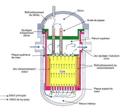
Figure 44: Main flow and core bypass flow in normal operation
