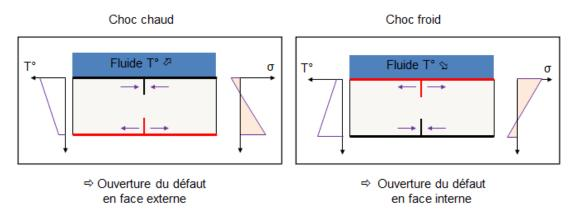
Figure 43: Effect of a thermal shock and pressure on a flaw perpendicular to the surface
