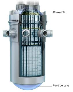
Figure 1: Representation of the Flamanville EPR reactor pressure vessel Closure head Bottom head
