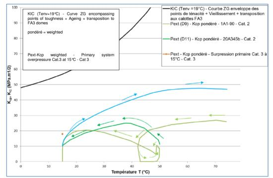
Figure A2. : Figure A27.: Upper dome - 10 mm flaw in outer surface - Indexing temperature of 19°C - Change of stress intensity factor and toughness as a function of temperature for designbasis situations
