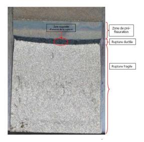
Figure 40: Fracture surface typical of a CT25 specimen tested at 50°C and 330°C
