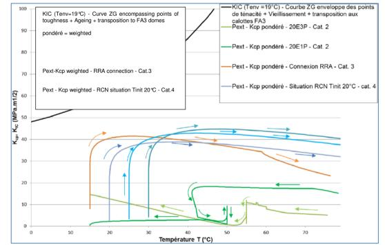
Figure A3. : Figure A27.: Lower dome - 10 mm flaw in outer surface - Indexing temperature of 19°C - Change of stress intensity factor and toughness as a function of temperature for design-basis situations
