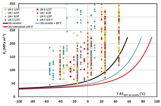
Figure 37: Positioning of fracture toughness data from the test programme in relation to the RCC-M curve [13]
