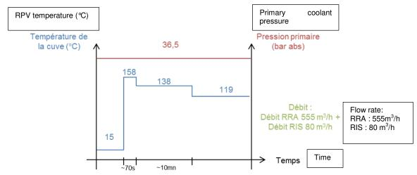
Figure A4: Fluid temperature and primary coolant pressure profiles applicable at RPV lower head in case of connection of an RIS-RA train in RA mode with Tcore exit > 135°C (case 2)
