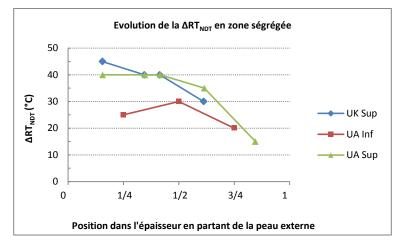
Figure 32: Evolution of the RT<sub>NDT</sub> shift in segregation zone in the thickness of the scale-one replica domes
