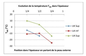
Figure 28: Evolution of  $T_{68J}$  as a function of the position in the thickness of the scale-one replica domes
