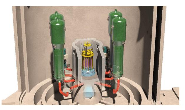
Figure A12 : The reactor pressure vessel (RPV) in the reactor building
