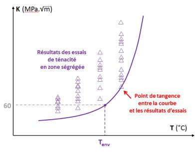
Figure 18: Principle for determining T<sub>env</sub>
