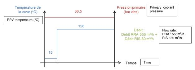
Figure A3 : Fluid temperature and primary coolant pressure profiles applicable at RPV lower head in case of connection of an RIS-RA train in RA mode with  $T_{core exit} > 135^{\circ}C$  (case 1)
