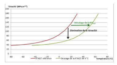
Figure 5: Effect of transition temperature shift on toughness
