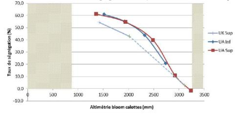
Figure 21: Evolution of maximum segregation ratio (carbon content relative to median acceptance value)
