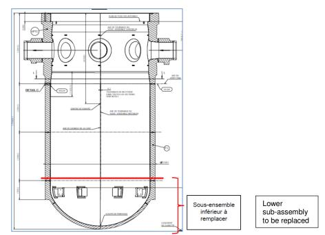
Figure A13 : Cutting the lower section of the RPV in order to replace the dome
