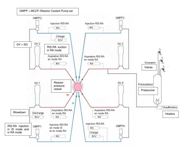
Figure A2 : Diagram of the RIS-RA system connected to the primary cooling system
