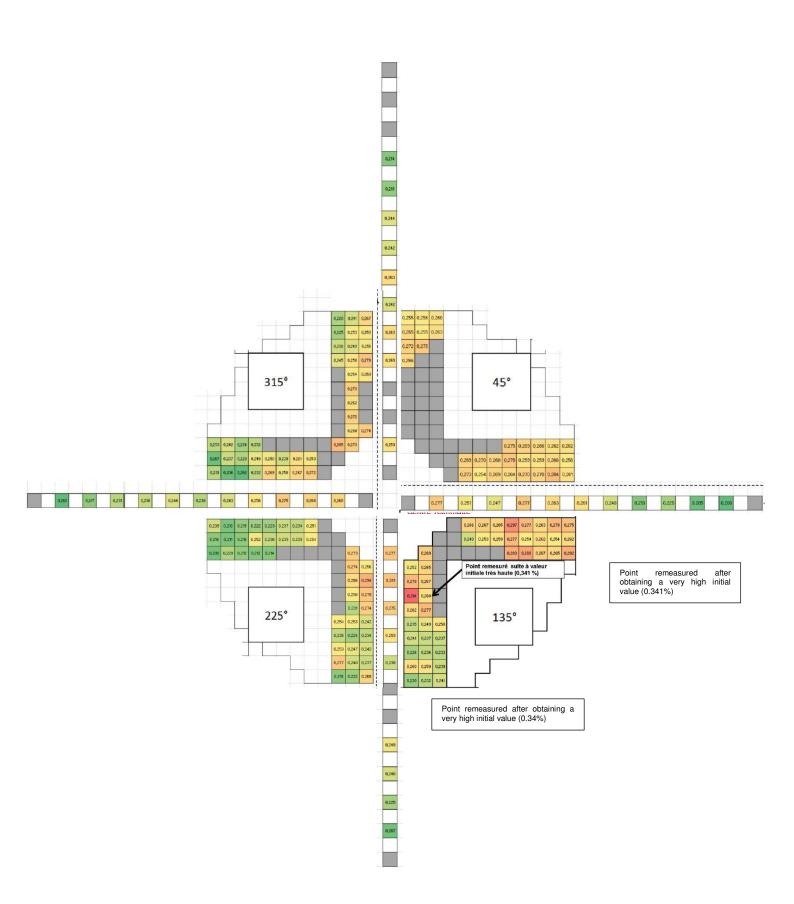
Figure A21. : Illustration of the most segregated zone on external surface of FA3 upper dome (OES measurements - Areva NP's device) Measurement pitch 30 mm x 30 mm
