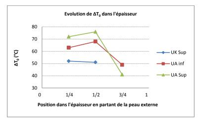
Figure 35: Evolution of the T<sub>0</sub> shift between the segregation zone and the acceptance zone in the thickness of the UK, UA domes
