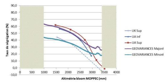
Figure 23: Evolution of the maximum carbon content – comparison of domes with postprocessed, upper bound and lower bound MOPPEC data
