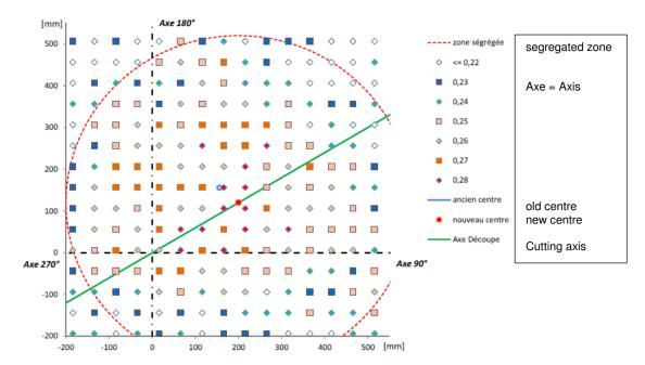
Figure A18 : Illustration of the most segregated zone on external surface of UA lower dome (OES measurements - contractor's device) Measurement pitch 50 mm x 50 mm
