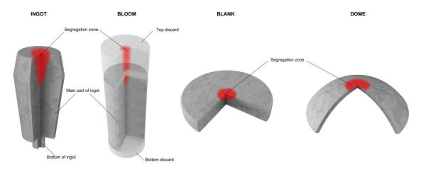
Figure 2: Position of positive macrosegregation during forging
