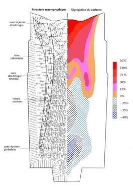
Figure 3: Structure and carbon segregation in a conventional ingot
