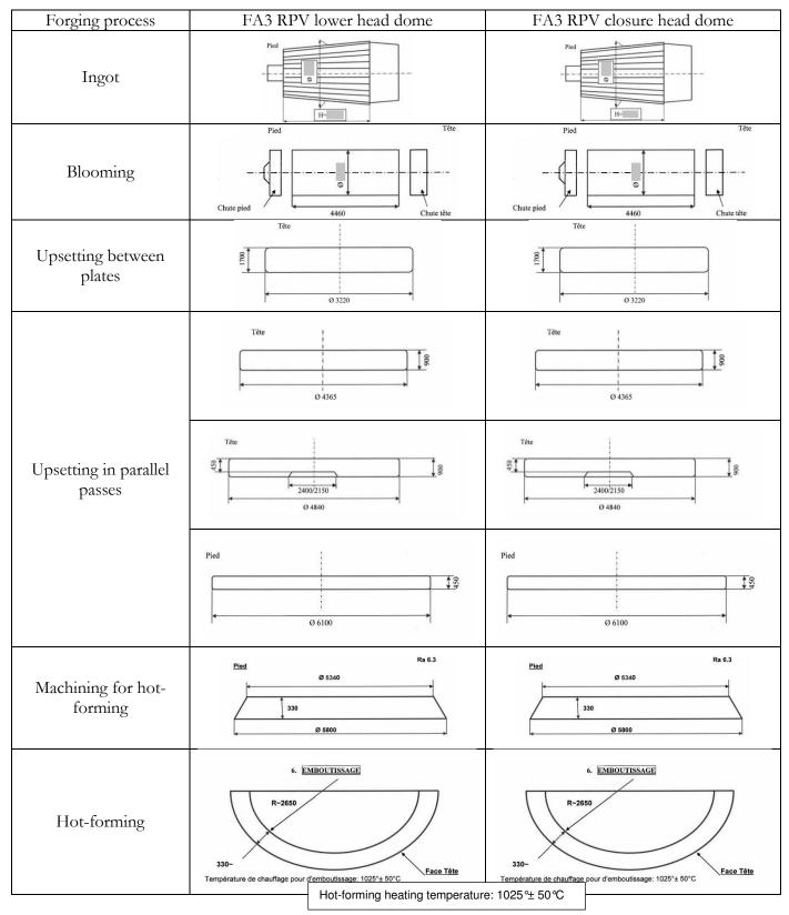
Figure A15 : Forging process for the upper and lower domes of the Flamanville A3 reactor
