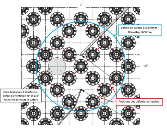
Figure 49: Central part of the Flamanville EPR reactor pressure vessel seen from above – zone to be examined and positions of flaws looked for Limit of zone to be examined: Diameter 1600 mm
