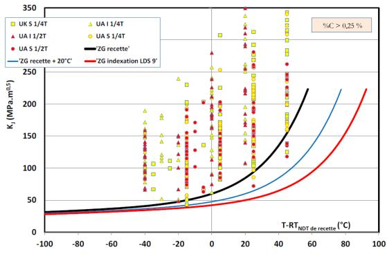
Figure 38: Positioning in relation to the RCC-M curve of the toughness data from specimens with carbon contents greater than or equal to 0.25 % [13]
