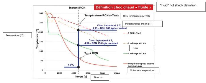
Figure A5: Principle of the Areva NP approach to characterise the category-3 hot shock resulting from the RCN situation following a small break
