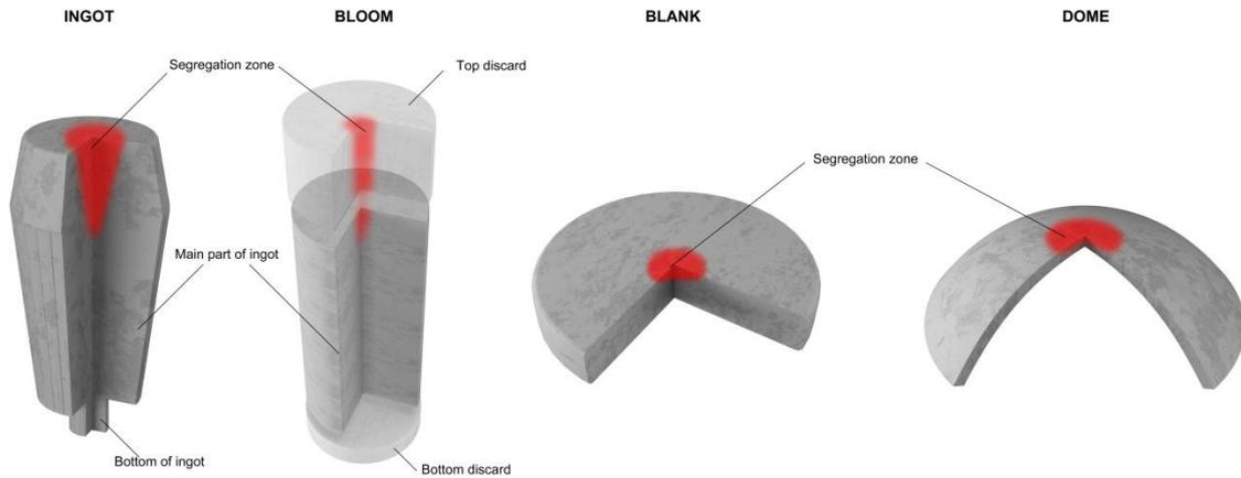
Figure 2: Position of positive macrosegregation during forging
