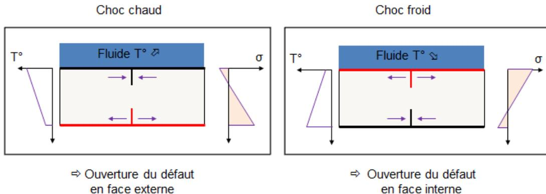
Figure 43: Effect of a thermal shock and pressure on a flaw perpendicular to the surface
