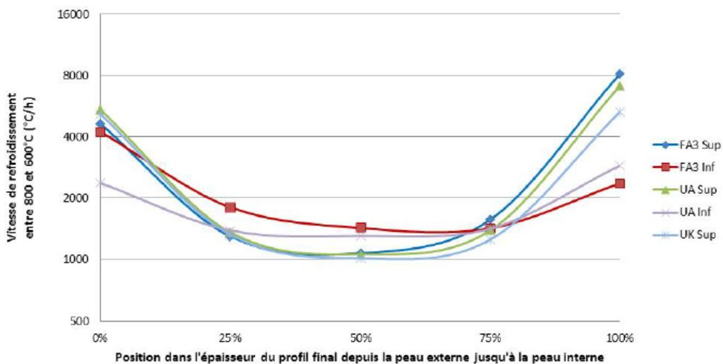
Figure 16: Results of numerical simulations of quenching operations: evolution of cooling rate during quenching versus thickness of domes
