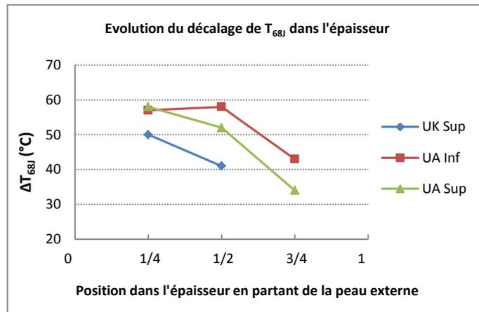
Figure 29 : Evolution of shift in  $T_{68J}$  as a function of the position in the thickness of the scale-one replica domes
