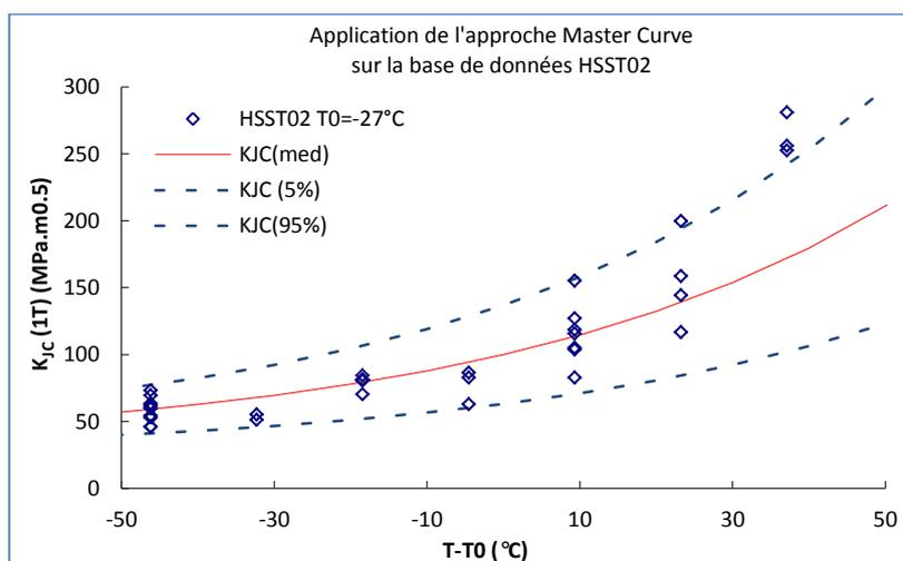
Figure 33: Application example given by the rapporteur for the Master Curve approach
