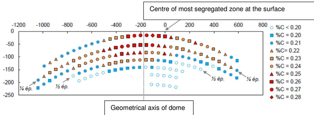
Figure A23. : Carbon content in thickness of UK upper dome
