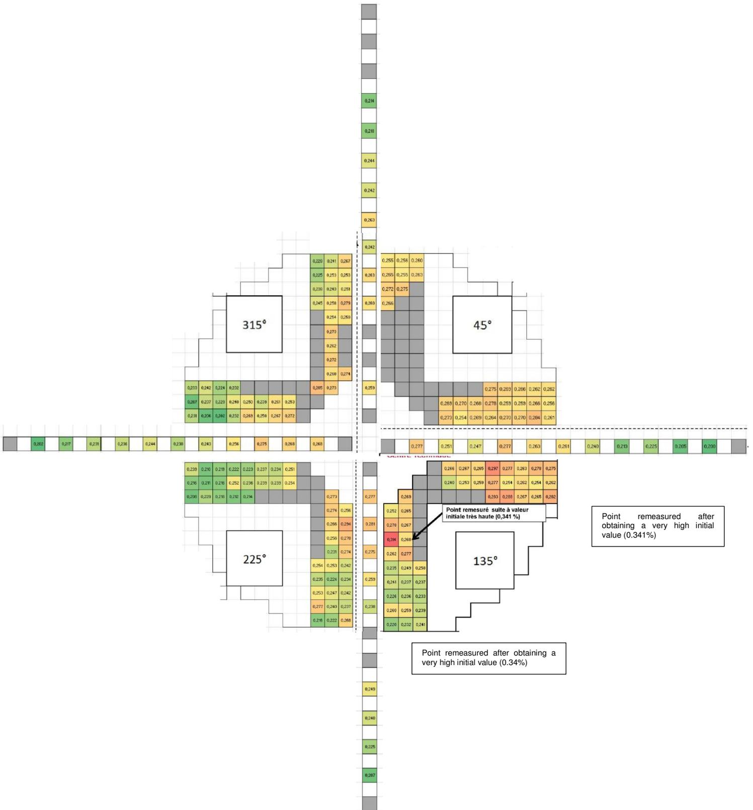
Figure A21. : Illustration of the most segregated zone on external surface of FA3 upper dome (OES measurements - Areva NP's device)
