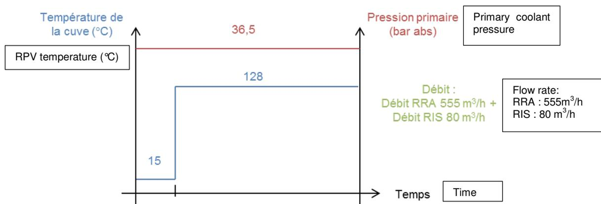
Figure A3 : Fluid temperature and primary coolant pressure profiles applicable at RPV lower head in case of connection of an RIS-RA train in RA mode with  $T_{\text{core exit}} > 135^{\circ}\text{C}$  (case 1)
