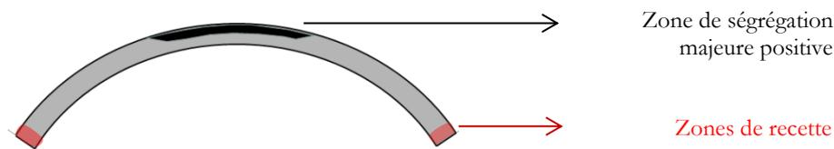
Figure 8: Cross-section of a dome - identification of acceptance and segregation zones
