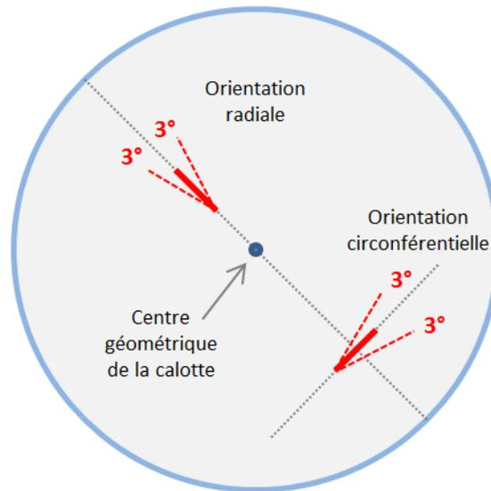
Figure 48: Orientation of flaws sought – dome top view
