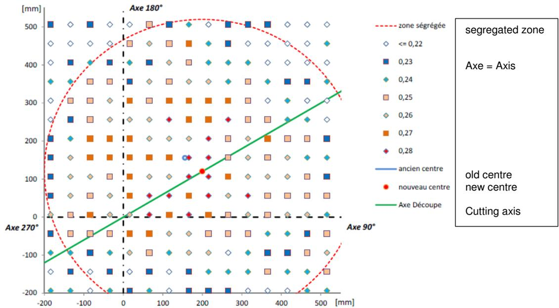
Figure A18 : Illustration of the most segregated zone on external surface of UA lower dome (OES measurements - contractor's device)
