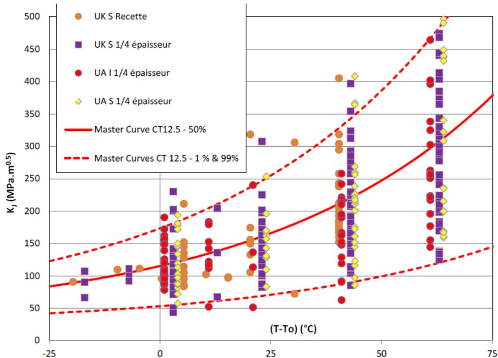
Figure 36: Positioning of the fracture toughness data for the specimens sampled at one-quarter thickness of the scale-one replica domes [13]
