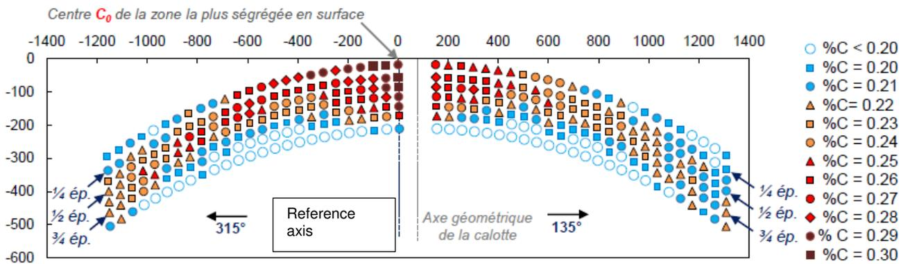
Figure A25. : Carbon content in thickness of UA upper dome
