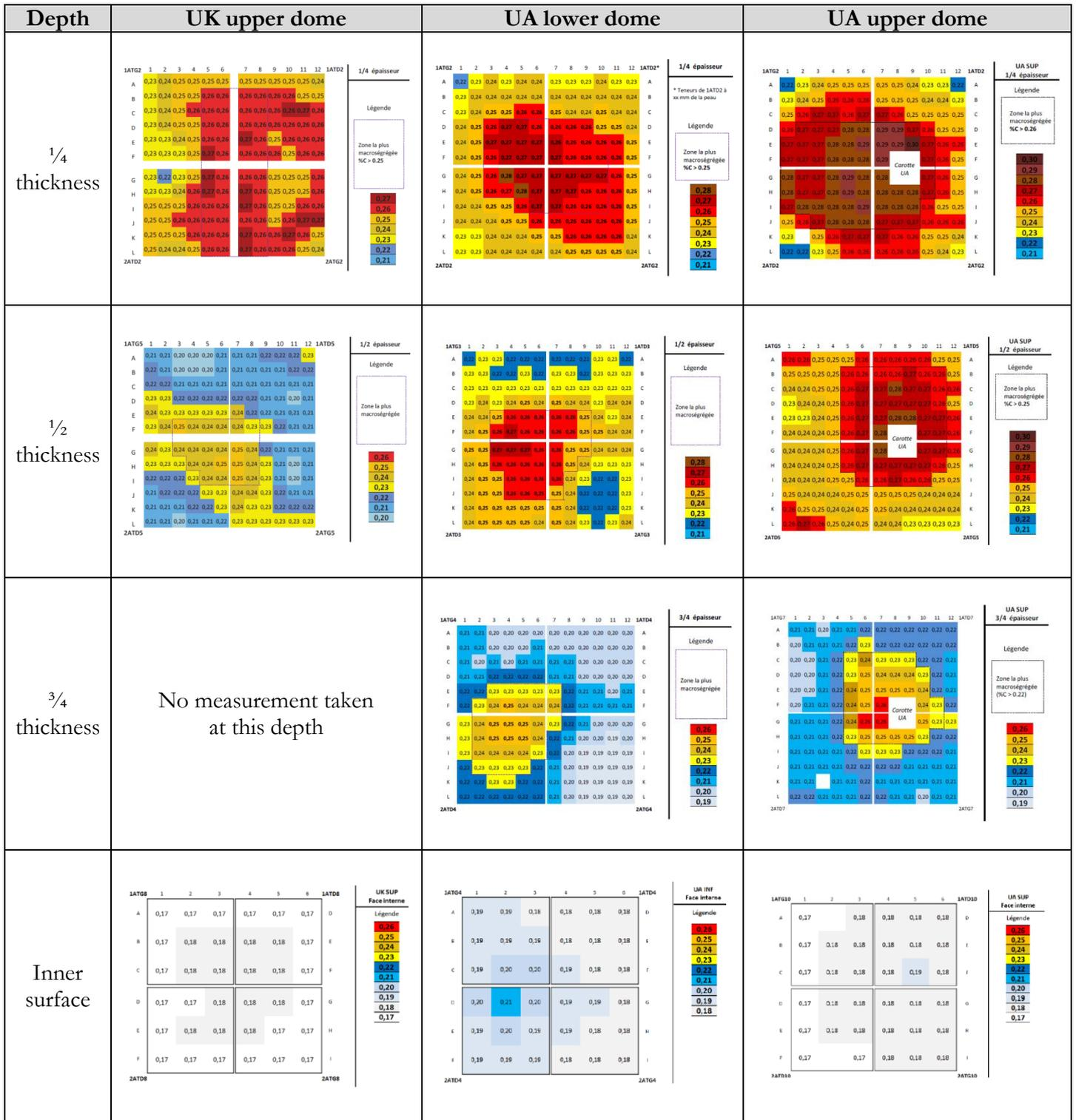
Figure A26 : Synthesis of carbon content mappings by depth (IRC measurements)
