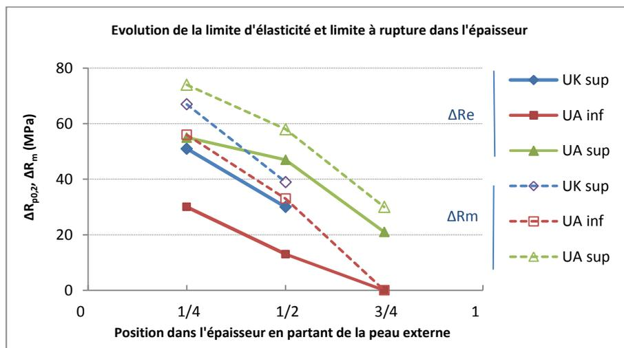
Figure 26: Shift in yield strength and ultimate tensile strength at 330°C in the segregation zone by comparison with the acceptance zone, as a function of position in the thickness
