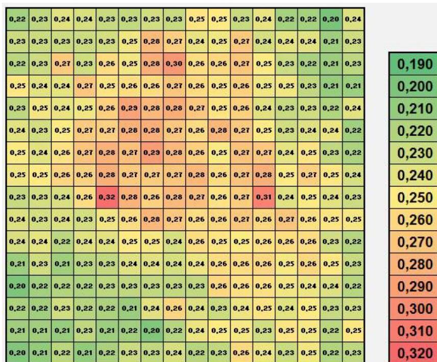
Figure A19 : Illustration of the most segregated zone on external surface of UA lower dome (OES measurements - Areva NPs device)
