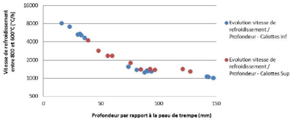
Figure 15: Results of numerical simulations of quenching operations: evolution of cooling rate during quenching versus distance to the surface
