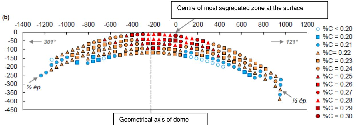
Figure A24. : Carbon content in thickness of UA lower dome
