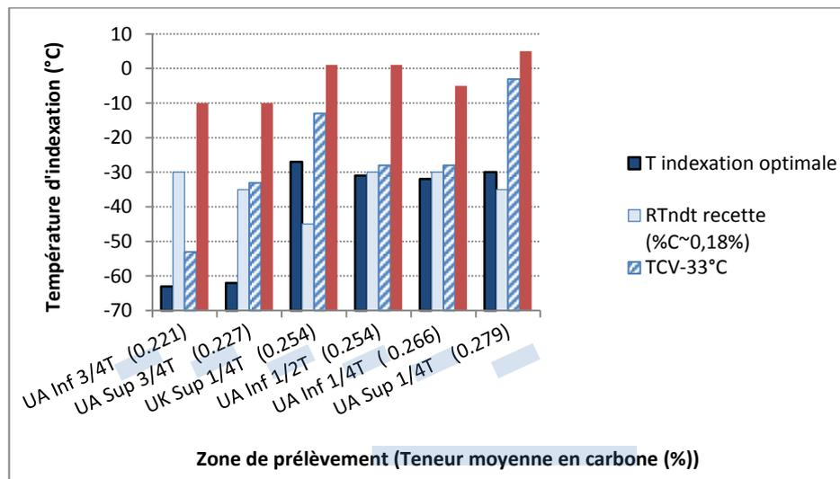
Figure 42: Comparison of the various index temperatures of the RCC-M curve examined in the light of the average carbon content measured on specimen<sup>34</sup>, at comparable quenching rate (~1300-1400°C/h)
