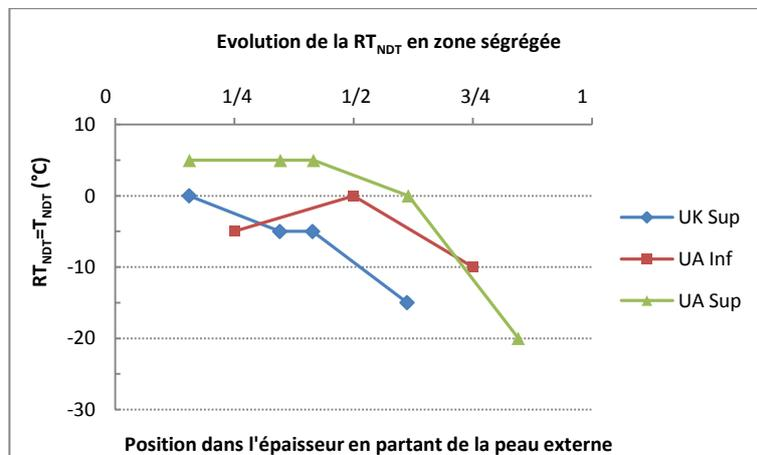
Figure 31: Evolution of the RT<sub>NDT</sub> in segregation zone in the thickness of the scale-one replica domes
