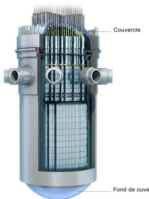
Figure 1: Representation of the Flamanville EPR reactor pressure vessel
