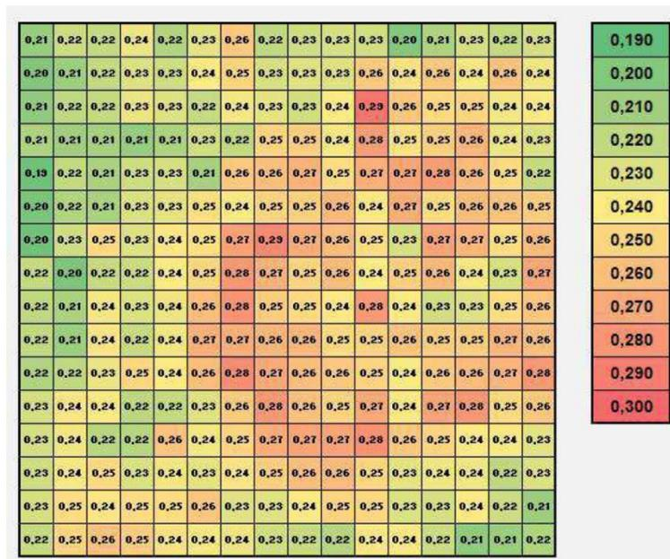
Figure A17 : Illustration of the most segregated zone on external surface of UK upper dome (OES measurements - Areva NP's device)
