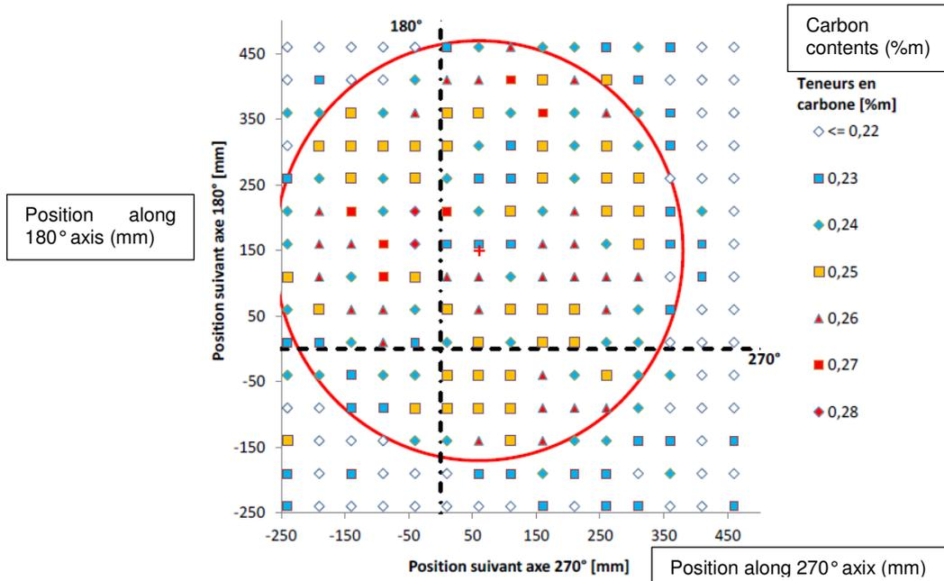
Figure A16 : Illustration of the most segregated zone on external surface of UK upper dome (OES measurements - contractor's device)
