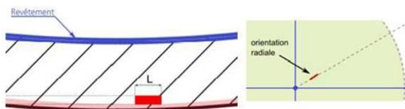
Figure 46: Radially oriented flaw
