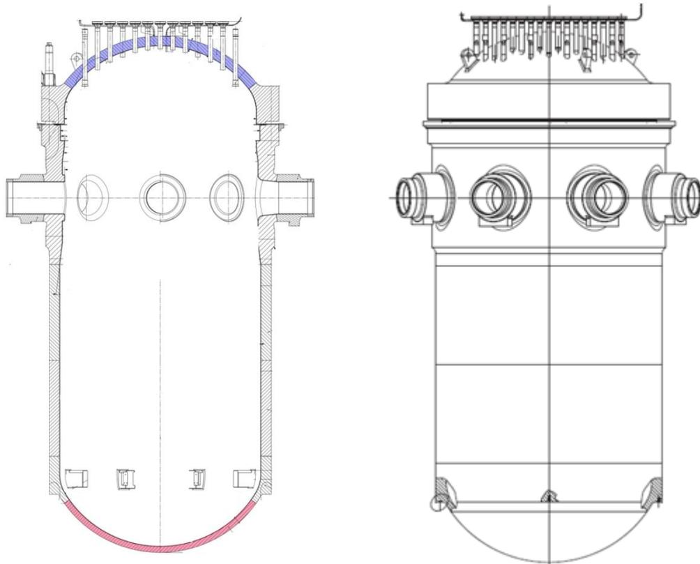
Figure A1. : Diagrams and components of the Flamanville EPR reactor pressure vessel
