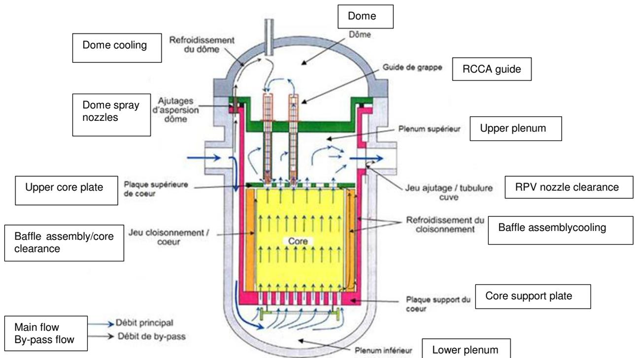
Figure A10 : Core main flow and by-pass flow in normal operation
