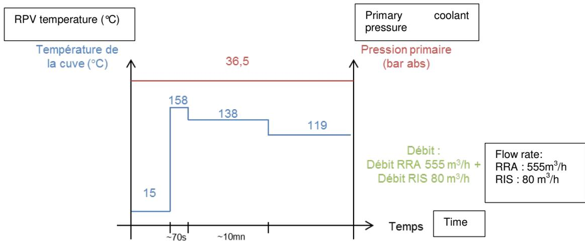
Figure A4: Fluid temperature and primary coolant pressure profiles applicable at RPV lower head in case of connection of an RIS-RA train in RA mode with Tcore exit > 135°C (case 2)
