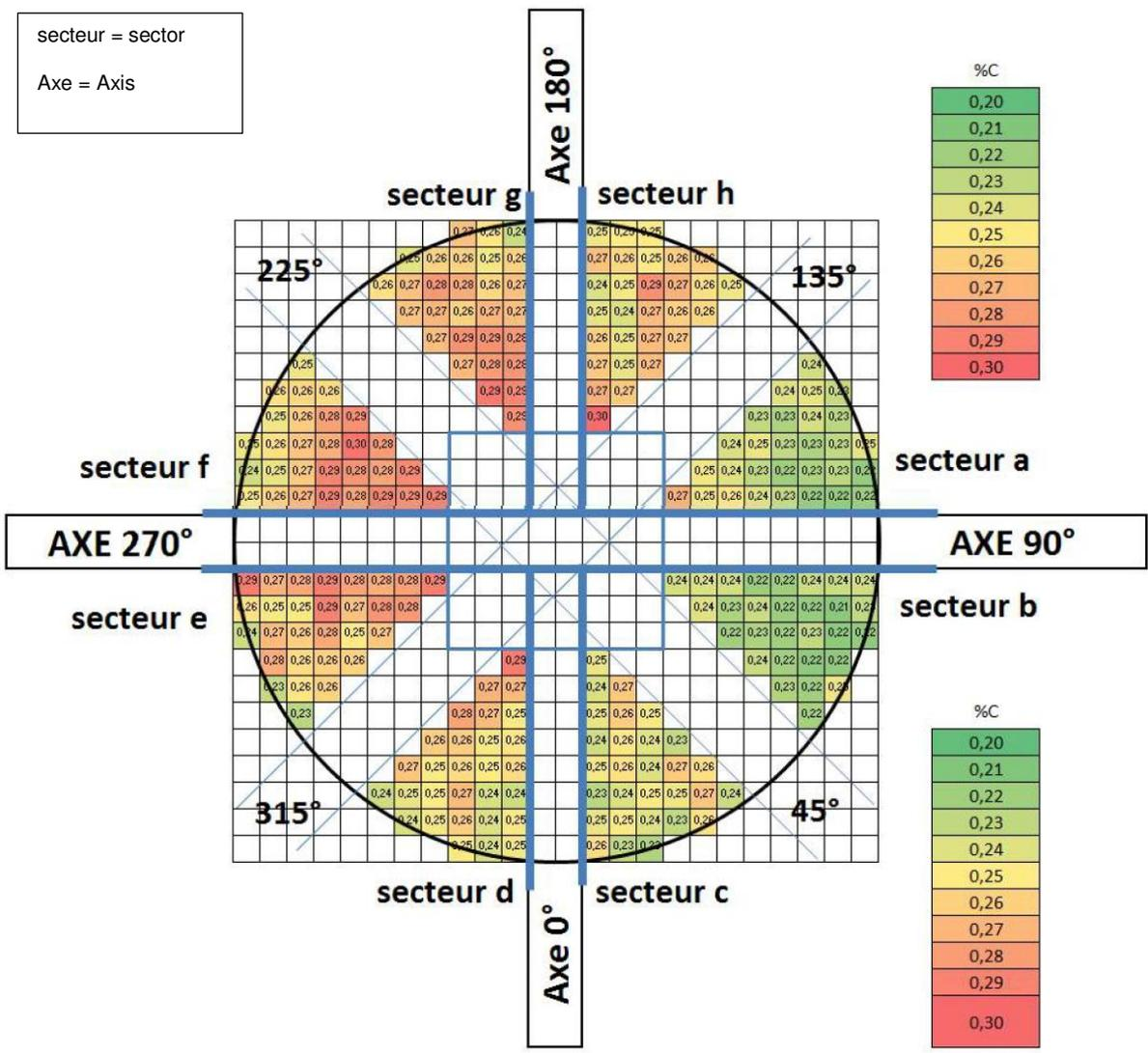
Figure A22. : Illustration of the most segregated zone on external surface of FA3 lower dome (OES measurements - Areva NPs device)
