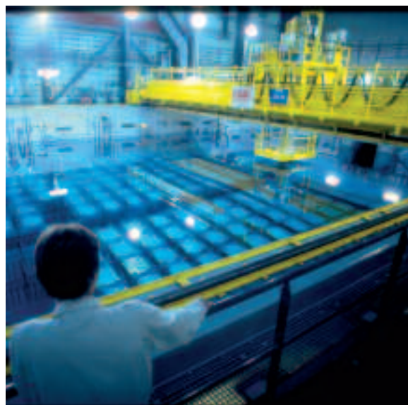
View of the spent fuel storage E pool in the Areva NC plant at La Hague (Manche département)
