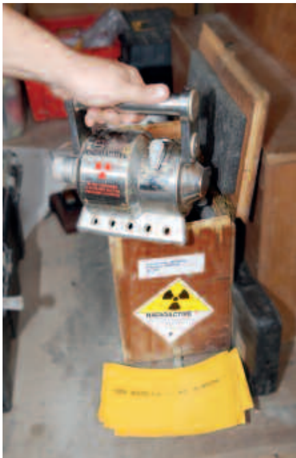
Gamma radiography appliance and its transport case
