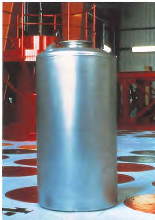
Package of high-level long-lived waste stored at COGEMA La Hague
