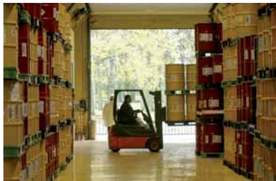
Storage shed for drums awaiting consignment to ANDRA (in yellow) or CENTRACO (in brown) after classification on the automated Camdices line. Solid radioactive waste management area in Saclay
