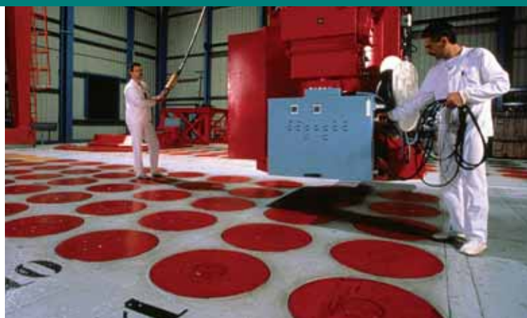
Storage shed at the vitrification workshop in Marcoule. The containers of vitrified waste are placed in cells at the site in Marcoule, for cooling inside ventilated pits
