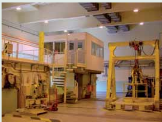
Cadarache nuclear installation No. 37 (INB 37) - 500 tonnes pressure to compact LL-ILW waste
