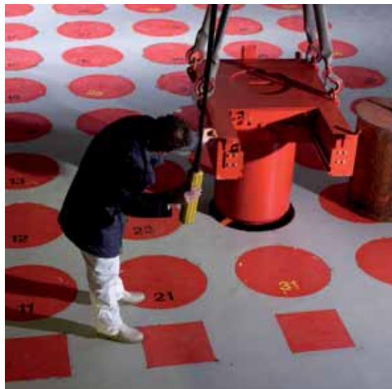
Waste management at the nuclear installation No. 72 (INB72) in Saclay - Storage shed in building 114. Each well is about ten meters deep; the highly radioactive drums are transported here in casks and covered with a concrete plug
