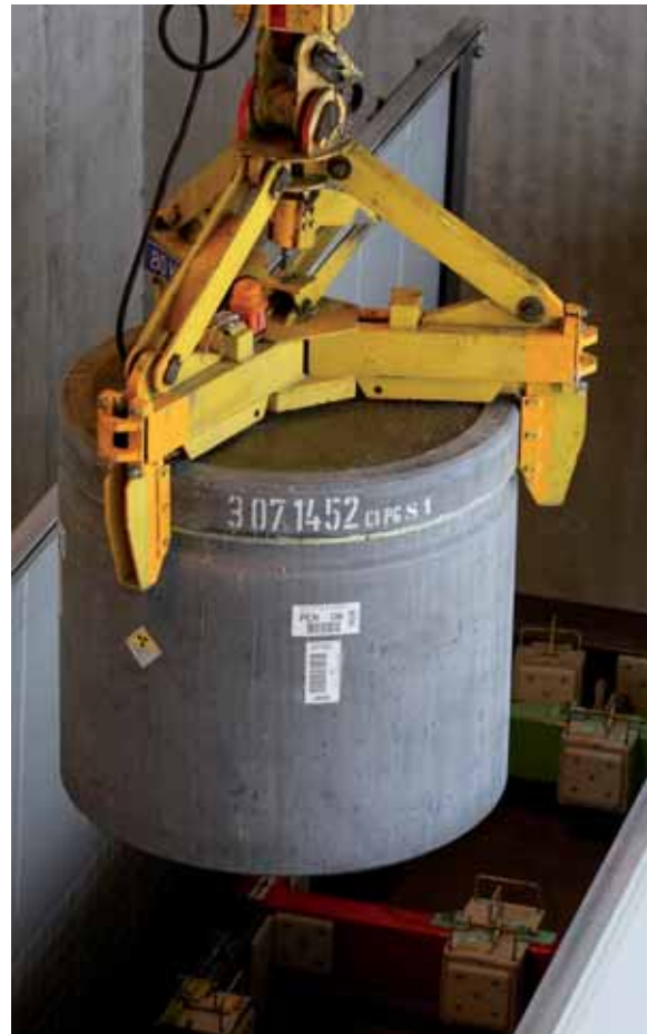
Unloading of a concrete container into a LILW cell in the Aube LILW storage facility (CSFMA)
