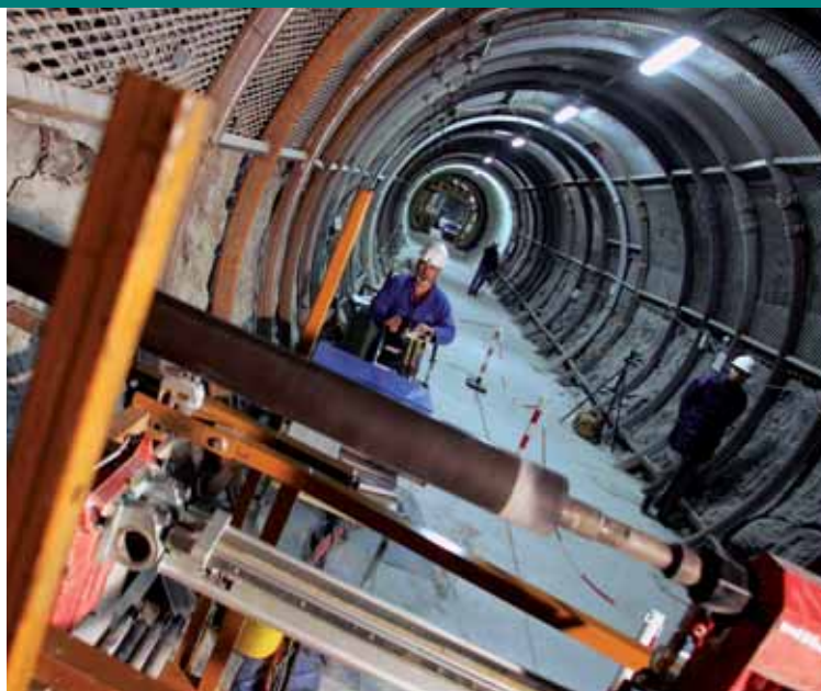
Drilling boreholes in a gallery at the Tournemire test station where the IRSN is carrying out its own research on deep geological disposal of waste.
