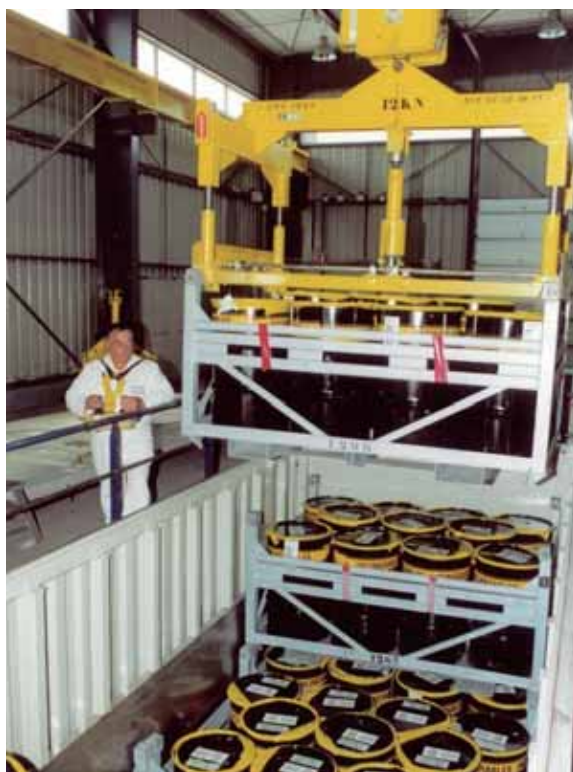
Loading drums of incinerable waste at the site in La Hague for the CENTRACO plant
