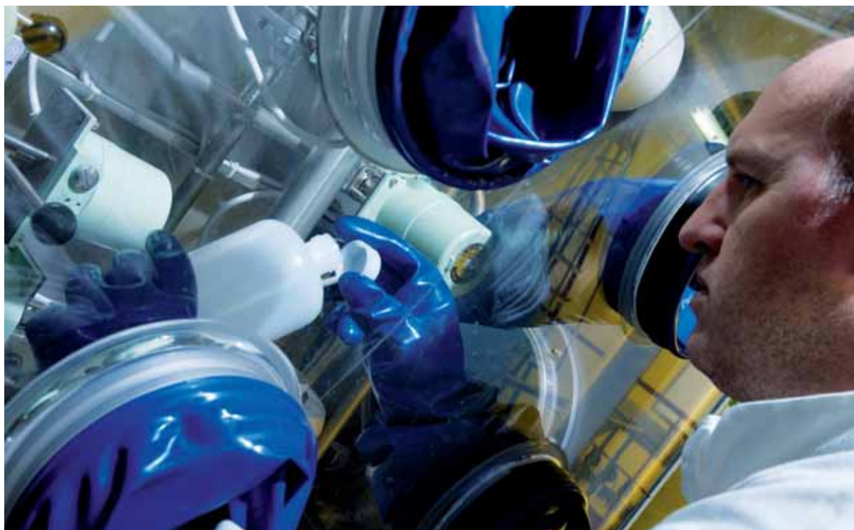
Building reservoir - nuclear installation No. 35 (INB 35) - taking samples for analysis using glove box. Nuclear installation No. 35 (INB 35) is a storage and treatment station for radioactive liquid effluents
