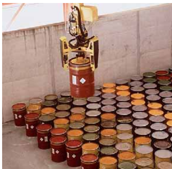
Placing metal drums in a disposal cell at the Aube LILW disposal facility
