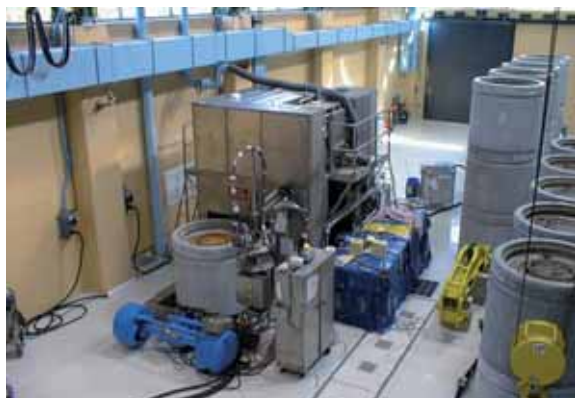
Mobile MERCURE units used for packaging ion exchanger resins in concrete hulls
