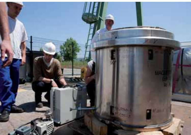
An IRSN engineer takes part in the resistance testing in an accident situation of a package design intended for transporting bituminized packages at the test station of TN International
