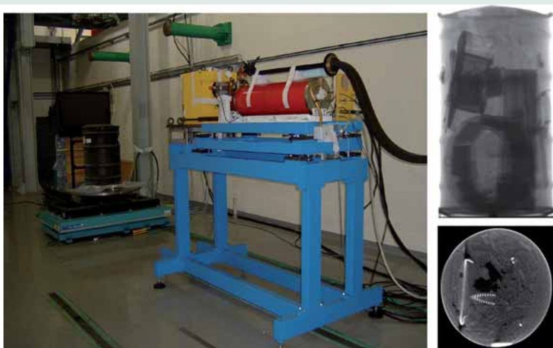
High-energy rapid imaging bench for physical classification of waste packages - Radiographic and tomographic imaging with linear electron accelerator and 2D wide field screen
