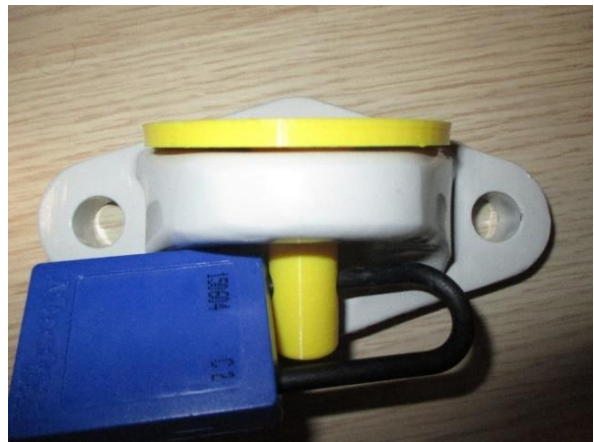
Figure 2: Tagged-out Tie-Off Point
