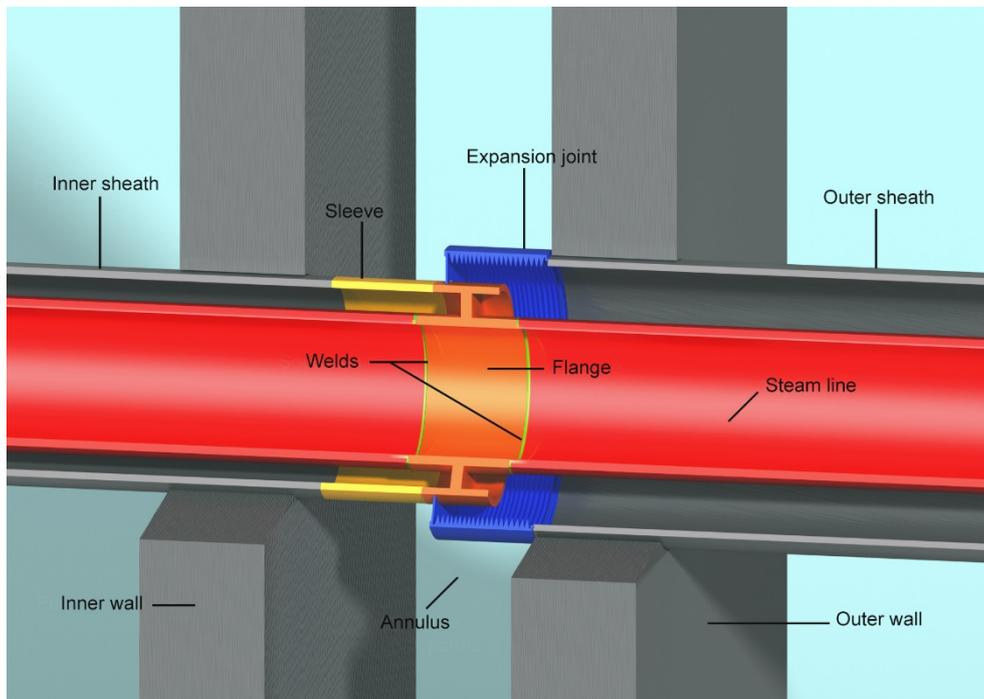
*Simplified cross-section of a penetration*
